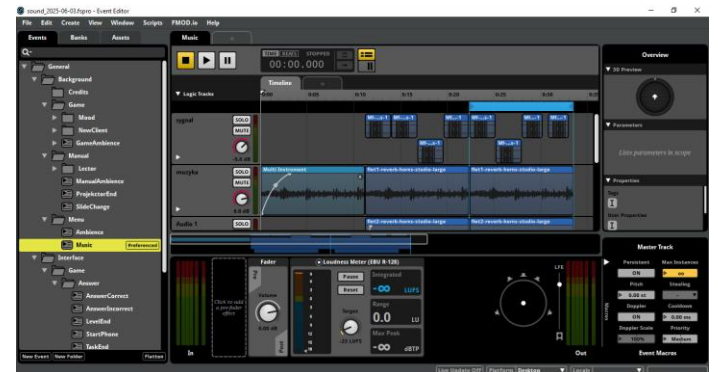
Fig. 5. Sound Jobs project in FMOD Studio showing the event hierarchy, parameter automation, and audio routing.
