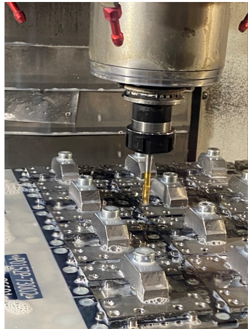
Fig. 7. Phasing with the help of a machining centre, source: own study.
