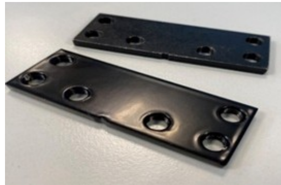
Fig. 9. Comparison of detail with powder and galvanised painting, source: own study
