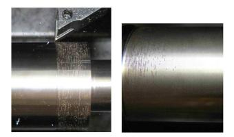
Fig. 22. Poor surface quality due to high wear of cutting plates
