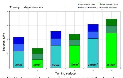
Fig. 15. Diagram of shear stresses in roughing grinding with a sharp wheel
