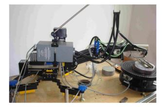
Fig. 8. Measurement system for residual stresses iXRD
