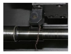
Fig. 4. Roughing with a circular plate of KNB
