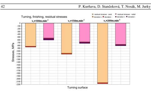
Fig. 12. Diagram of residual stresses in turning finishing
