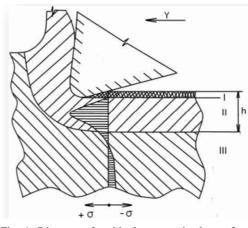
Fig. 1. Diagram of residual stresses in the surface layer under the influence of plastic deformation [1].
