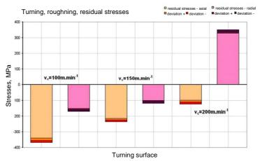
Fig. 10. Diagram of residual stresses in rough turning
