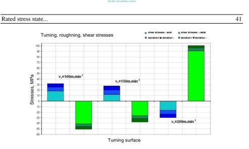
Fig. 11. Diagram of shear stress in rough turning
