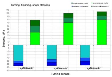
Fig. 13. Diagram of shear stresses in turning finishing
