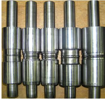
Fig. 2. Thorns on rolling bearing rings
