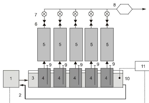
**Fig. 1.** The anaerobic digestion system: 1 – thermostated water heater, 2 – isolated water transfer tubes, 3 – heating jacket, 4 – biofermentors, 5 – biogas container with volumetric scale, 6 – cut-off valves, 7 – gas flow meters, 8 – gas analyzer, 9 – sample collection tubes, 10 – thermometer, 11 – control unit (Adamski et al., 2009)
