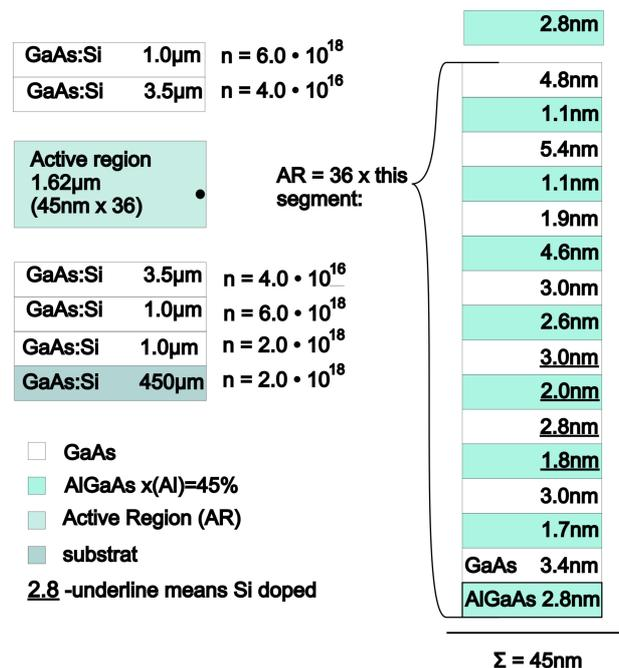
Fig. 1. Layer sequence in the Al<sub>0.45</sub>Ga<sub>0.55</sub>As/GaAs laser structure
