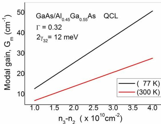
Fig. 8. Modal gain vs. inversion for different temperatures
