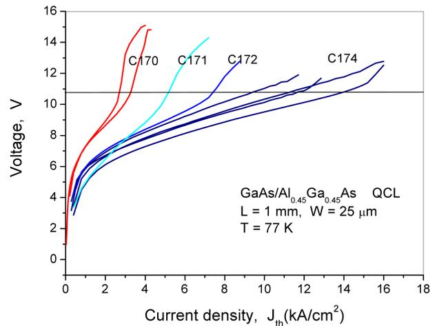
Fig. 5. Voltage-current characteristics for a set of  $\text{Al}_{0.45}\text{Ga}_{0.55}\text{As}/\text{GaAs}$  QCLs with different injector doping level ( $\sim 0.4\text{--}2.2 \times 10^{12}\ \text{cm}^{-2}$  per period); the doping concentration increases from structure C170 to C174
