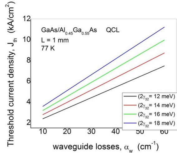
Fig. 9. Threshold current density vs. waveguide losses for different values of  $2\gamma_{32}$  parameter
