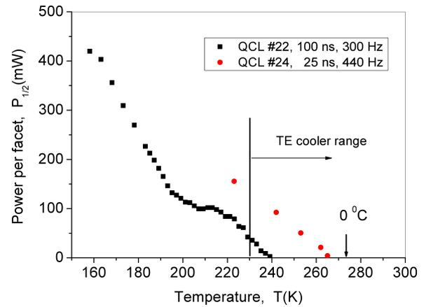
Fig. 10. Laser output versus temperature for two lasers operated at different pulse lengths
