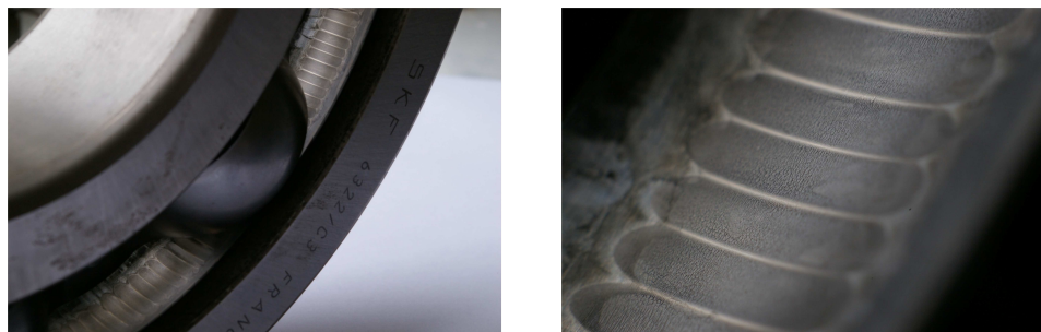
Fig. 3. Bearing race damages caused by EDM currents
