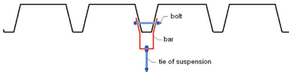
Fig. 2. Example of construction of connected to the corrugated sheet.
