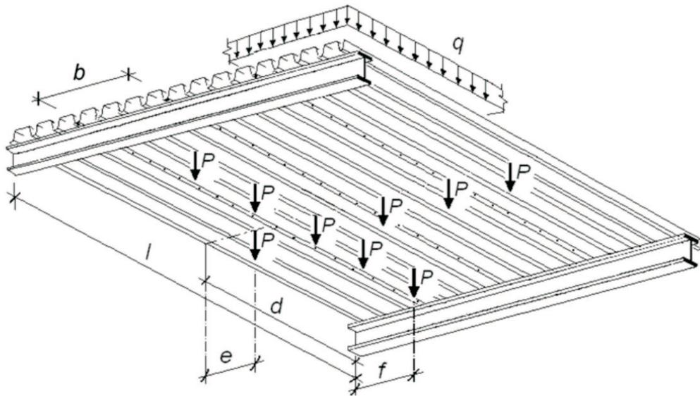
Fig. 1. Scheme of a corrugated sheet loaded by concentrated loads from local suspensions.
