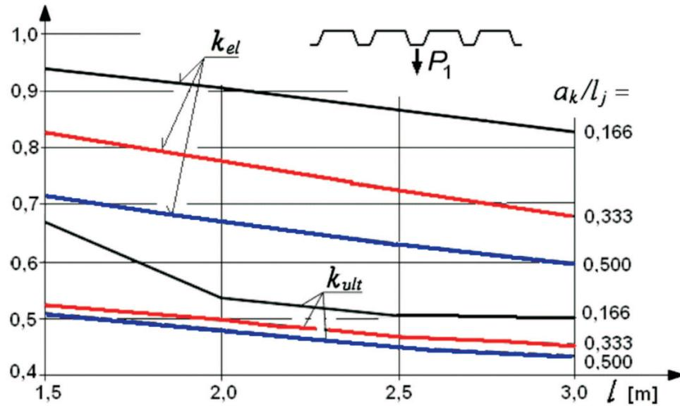
Fig. 6. Coefficients  $k_{el}$ ,  $k_{ult}$  for a fold under concentrated load  $P_1$  as functions of a span.
