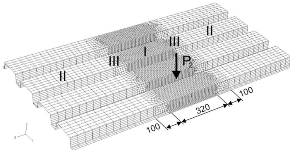
Fig. 4. Partition of finite elements for FEM model.
