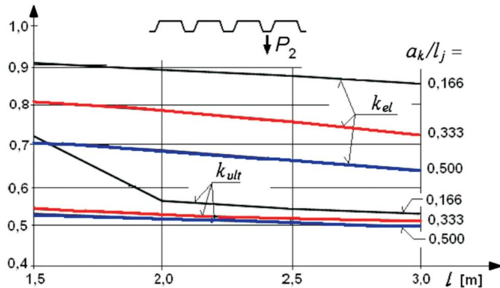
Fig. 7. Coefficients  $k_{el}$ ,  $k_{ult}$  for a fold under concentrated load  $P_2$  as functions of a span.
