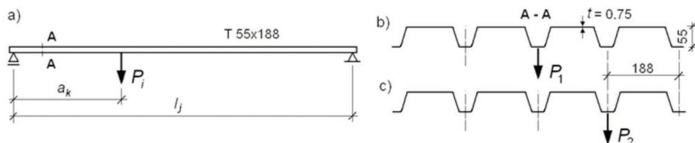
Fig. 3. Scheme of the tested corrugated sheets.
