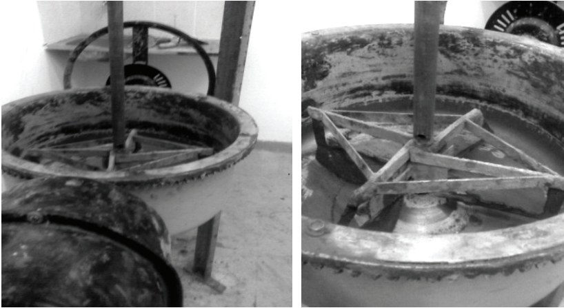
Fig. 2. The used concrete mixer.
