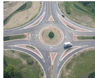
Fig. 3. Conventional Roundabouts with bypass lane
