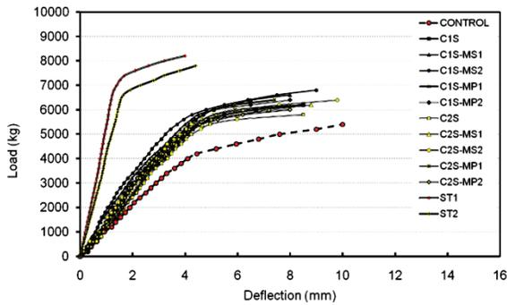
Fig. 17. Load-deflection relationships for all tested beams
