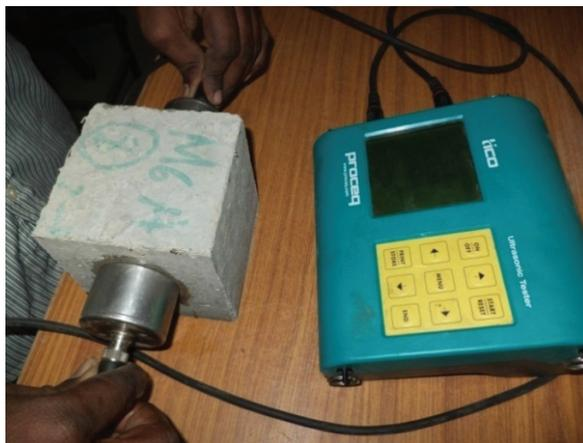
Fig. 4. Test set up for Ultrasonic Pulse Velocity
