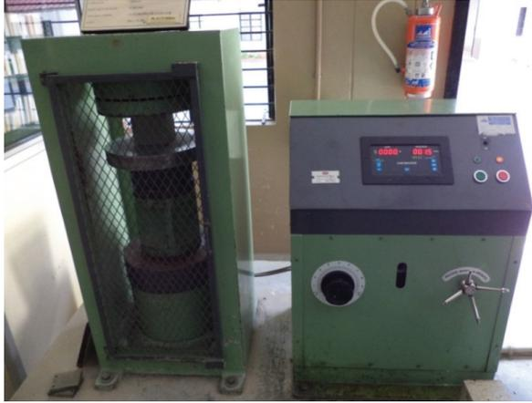
Fig. 3. Test set up for Compression testing machine
