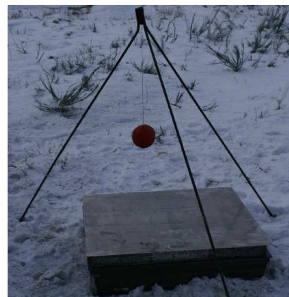
Fig. 3. A general view of the position of test panels loaded by large explosives
