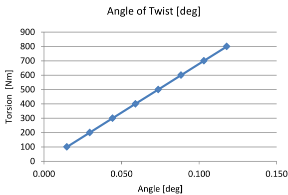
Fig. 6. Angle of twist of the propeller shaft modeled with tetrahedron linear and hexahedra FEM elements
