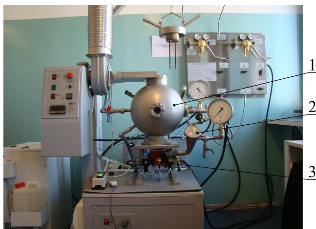
Fig. 1. Test apparatus to determination of explosion characteristics dust clouds: 1 – 20 dm 3 explosion-proof sphere, 2 – dust container, 3 – fast discharge valve
