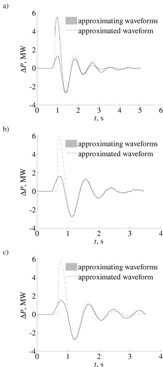
Fig. 3. Measured instantaneous power deviation waveforms of unit no 5 in Rybnik Power Plant for duration of the step disturbance:  $t_{imp} = 290$  ms (a),  $t_{imp} = 343$  ms (b) and  $t_{imp} = 420$  ms (c)
