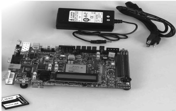
Figure 7. FPGA Spartan 3E board.
