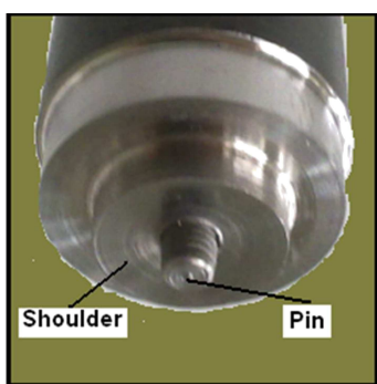
Fig. 2. Mixer pin used in FSW
