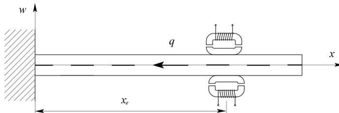
Figure 1. Analyzed system – Leipholz column with electromagnetic actuators
