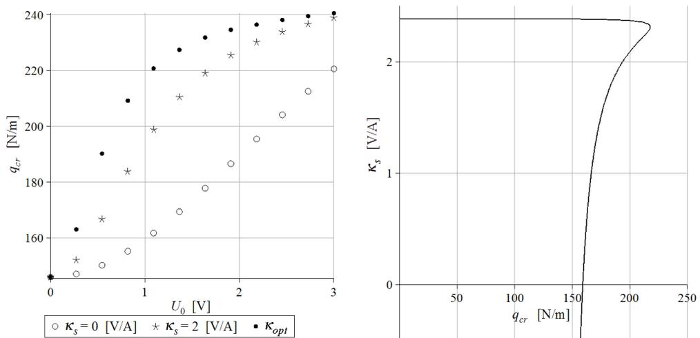
Figure 4. Critical compressive load for the simple control depending on the current and without active control (on the left) and the relation between this load and the control for  $U_0 = 1$  V (right),  $x_e = 0.33L$ , air.
