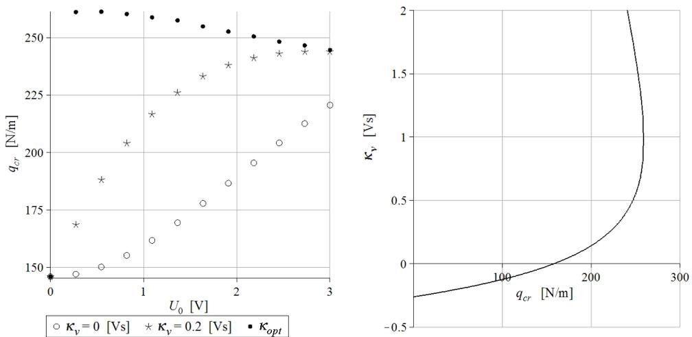
Figure 3. Critical compressive load for the control depending on velocity and without active control (on the left) and the relation between this load and the control for  $U_0 = 1$  V (right),  $x_e = 0.33L$ , air.
