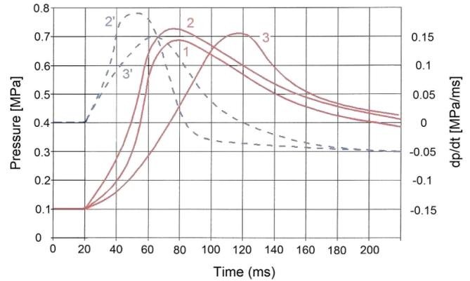
Fig. 13. Traces of combustion pressure of propane-air mixture: 1 – one jet flowing from the pre-ignition chamber at  $\phi = 1.95$  to the main combustion chamber filled by a mixture at  $\phi = 0.7$ ; 2 – three jets under the same conditions as in 1; 3 – flame initiated directly in the main combustion chamber filled by a mixture at  $\phi = 1.05$ ; 2' – rate of pressure increase  $dp_2/dt$ ; 3' – rate of pressure increase  $dp_3/dt$
