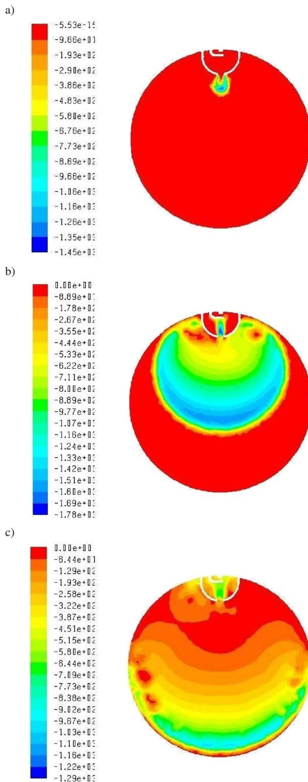
Fig. 2. Contours of net reactions rate of  $\text{C}_3\text{H}_8$  [ $\text{kg}/(\text{m}^3 \text{ s})$ ] at time: a) 0.01, b) 0.02 and c) 0.026 s after start of ignition with one outflow hole of rich mixture chamber
