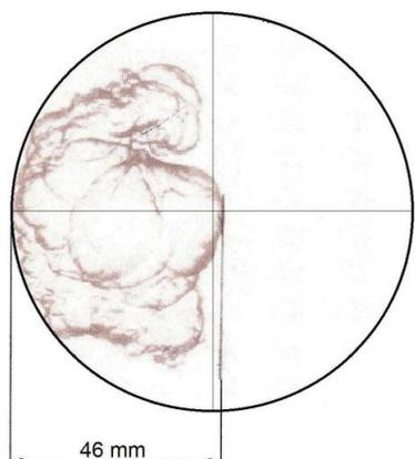
Fig. 16. The shape of the flame front initiated by three jets flowing from the pre-ignition chamber at  $\phi = 1.95$  to the main combustion chamber at  $\phi = 0.7$  with a time delay of 20 ms. Flame displacement marked in real value
