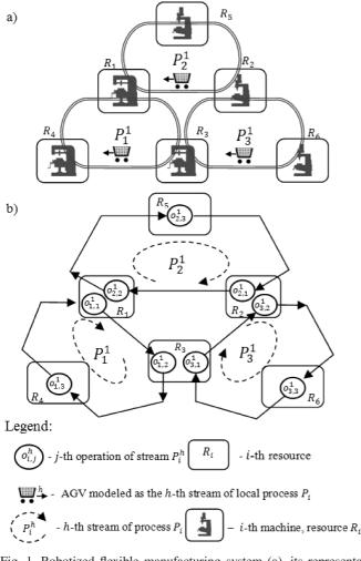
Fig. 1. Robotized flexible manufacturing system (a), its representation in the form of SCCP with three processes (b)
