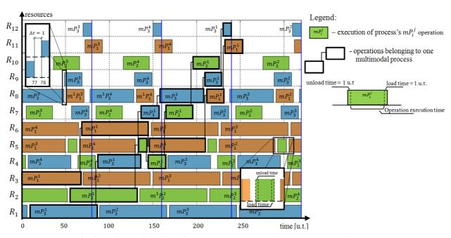
Fig. 6. Cyclic schedule of multimodal processes representing accepted production plan
