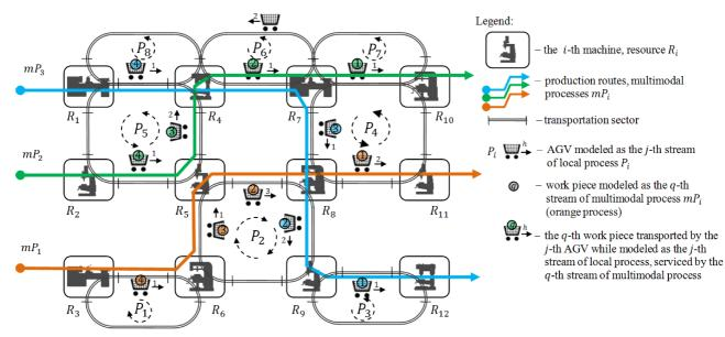
Fig. 4. System of stream production with AGV transport sub-system
