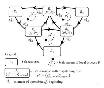
Fig. 8. Example of SCCP described by dispatching rules:  $\sigma_1^0 = (P_2^1, P_3^1) \sigma_2^0 = (P_2^1), \sigma_3^0 = (P_2^1, P_1^1), \sigma_4^0 = (P_1^1) \sigma_5^0 = (P_3^1, P_1^1), \sigma_6^0 = (P_3^1)$
