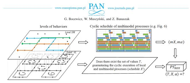
Fig. 7. Determination of parameters of SC structure for the system from Fig. 5 in top-down strategy
