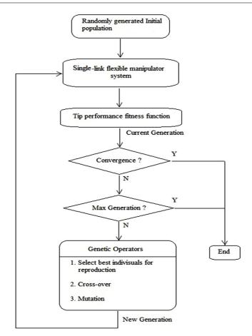
Figure 6. Genetic algorithm optimization process.
