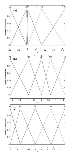
Figure 10. BFO optimized FLC membership functions: (a) E, (b) CE, (c) T.
