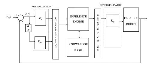
Figure 2. Structure of fuzzy logic controller.
