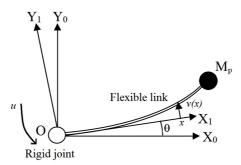
Figure 1. A single-link flexible manipulator.
