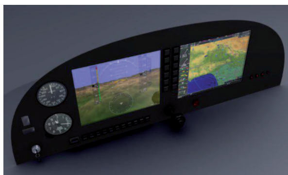
Fig. 4. Initial design of instrument panel
