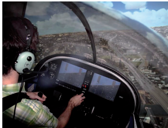
Fig. 3. Instrument panel with a dual PFD
