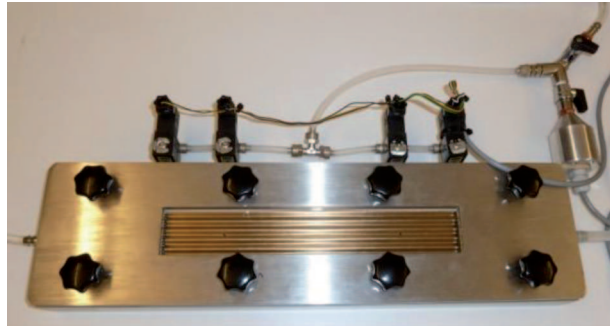
Fig. 12. Experimental model of the wavy channel. The corrugated bottom wall is visible through the top glass wall
