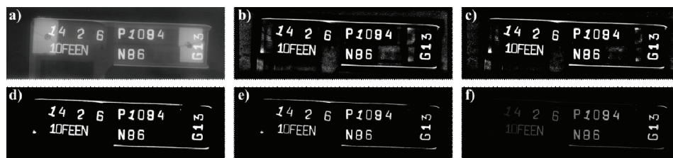
Fig. 5. Results of successive stages of letters extraction: a) fragment of radiographic image; b) image after thresholding using Sauvola algorithm; c) image after filtering; d) image after morphological closing; e) image after morphological eroding; f) image after indexation
