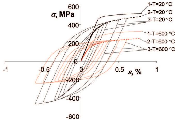
Fig. 11. Position of the graphs of static and cyclic strain obtained at the temperature of 20 and 600°C: 1 – static tension curve, 2 – cyclic strain curve, 3 – hysteresis loops
