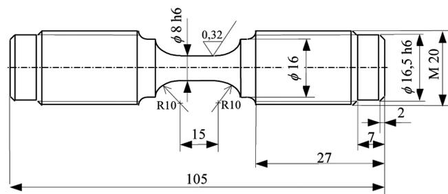
Fig. 1. The shape and dimensions of test samples used during the tests
