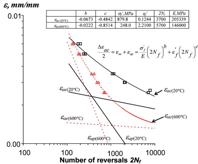
Fig. 12. Comparative graphs of fatigue life of the examined cast steel
