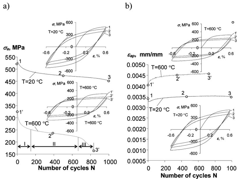
Fig. 7. Changes in the loop parameters at the level  $\epsilon_{ac} = 0.60\%$ : a)  $\sigma_a = f(n)$ , b)  $\epsilon_{ap} = f(N)$
