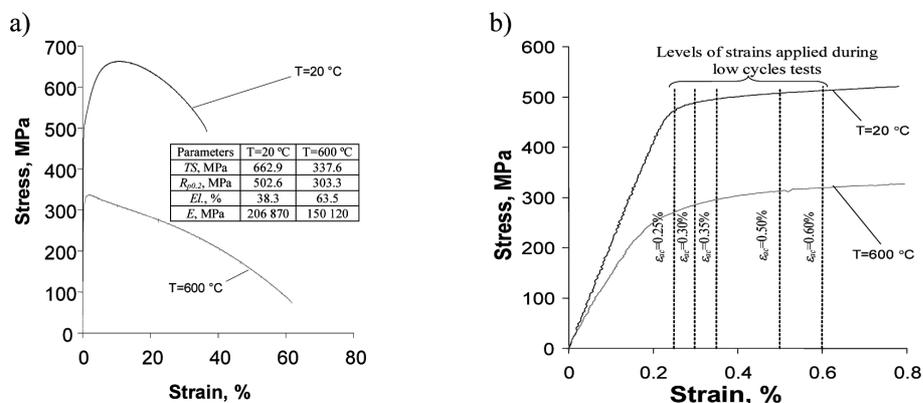
Fig. 4. Tension graphs: a) complete graphs, b) levels of strains applied during low cycle tests
