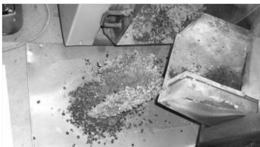
Fig. 2. Horizontal-feed wood pellet furnace, slag appears during hay pellet combustion
