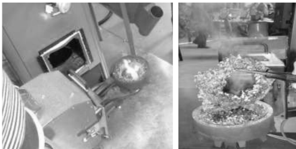
Fig. 3. Under-fed (retort) wood pellet furnace, slag can be observed during hay pellet combustion
