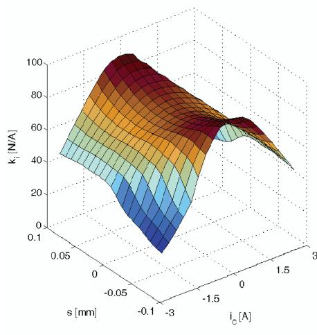
Fig. 9. Current gain vs. control current  $i_c$  and position of the rotor  $s$ , for  $\beta_2 = 25^\circ$
