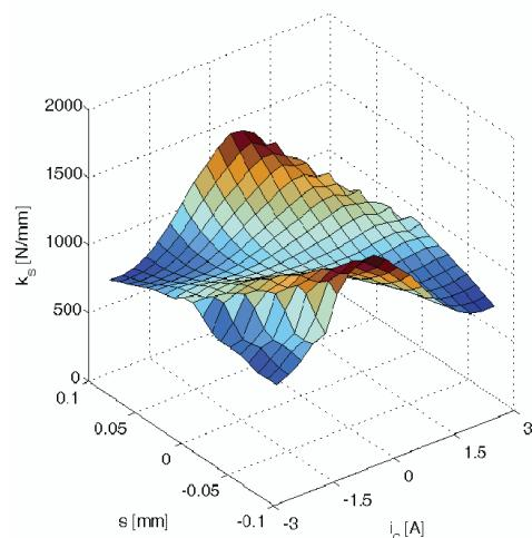
Fig. 10. Position stiffness vs. the control current  $i_c$  and position of the rotor  $s$ , for  $\beta_2 = 25^\circ$
