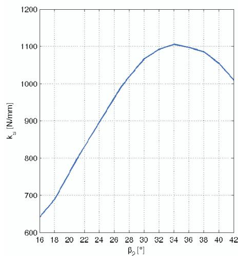
Fig. 7. Nominal position stiffness vs. the  $\beta_2$  angle
