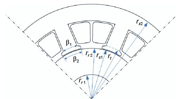
Fig. 3. Dimensions of the magnetic bearing actuator
