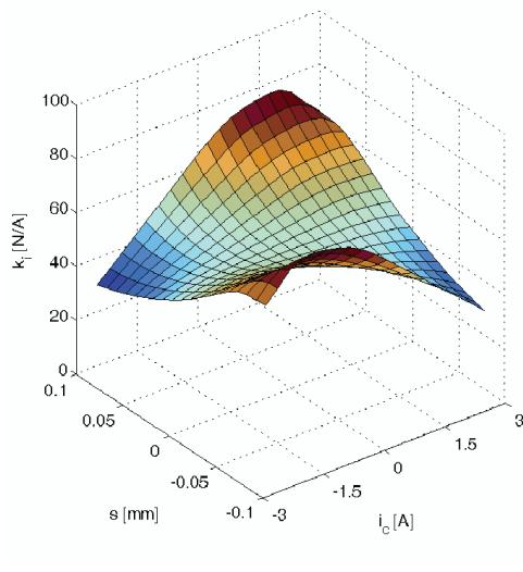
Fig. 4. Current gain value vs. the control current  $i_c$  and position of the rotor  $s$  for angle  $\beta_2 = 16^\circ$
