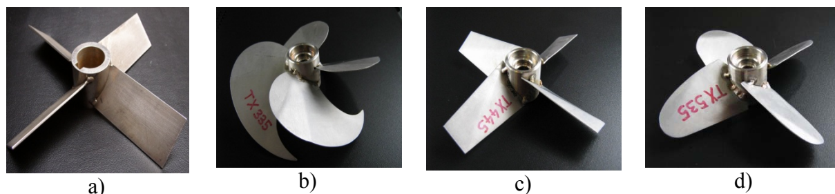
Fig. 1. Tested impellers: a) Pitched four-blade turbine (PBT), b) Techmix TX 335, c) Techmix TX445, d) Techmix TX535
