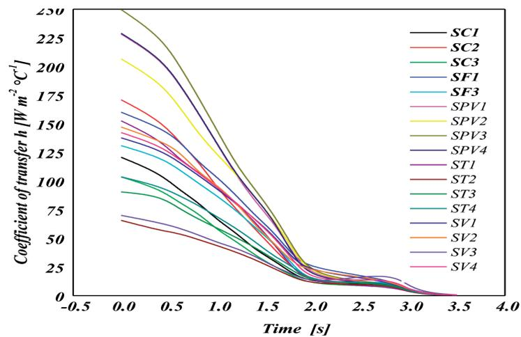
Fig. 13. Variation of heat-transfer coefficient ( $h$ ) of various surfaces for a ventilated disc in transient case (FG 15)
