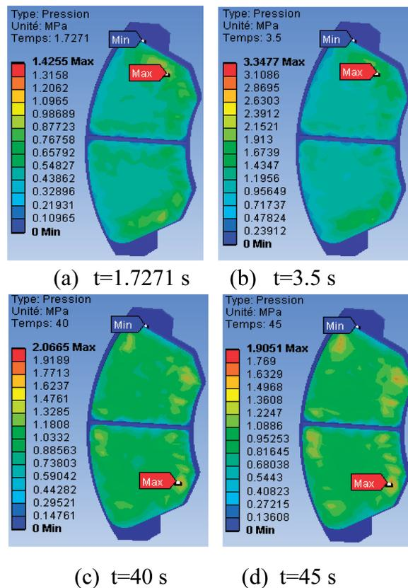
Fig. 23. Contact pressure distribution in the inner pad
