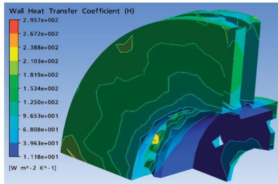
Fig. 11. Distribution of heat-transfer coefficient on a ventilated disc in the stationary case (FG 15)
