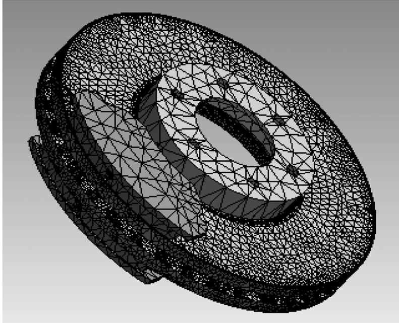
Fig. 20. Refined mesh of the model
