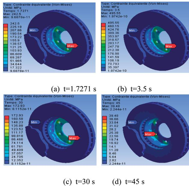
Fig. 22. Von Mises stress distribution
