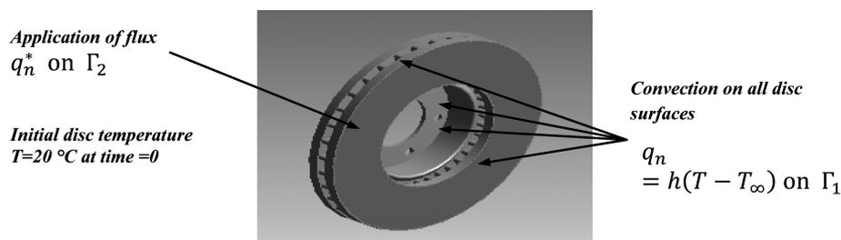
Fig. 2. Boundary conditions of the thermal analysis
