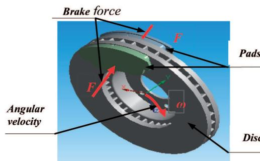
Fig. 1. Disc-pads assembly with forces applied to the disc
