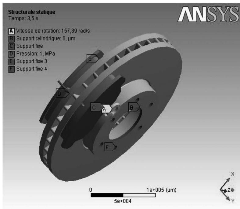
Fig. 19. Boundary conditions and loading imposed on the disc-pads
