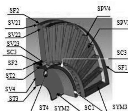
Fig. 7. Definition of surfaces of the ventilated disc
