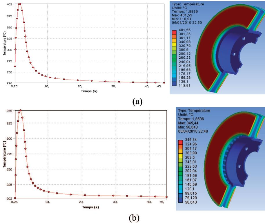
Fig. 17. Temperature distribution of a full (a) and ventilated disc (b) of cast iron(FG 15)
