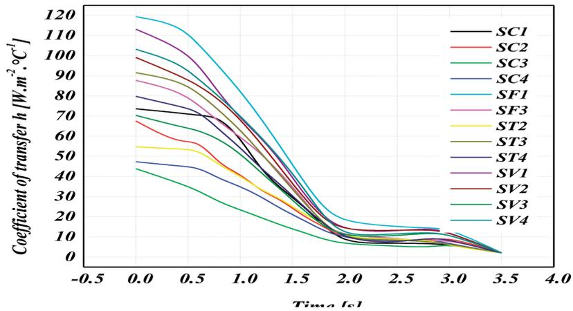
Fig. 12. Variation of heat-transfer coefficient ( $h$ ) of various surfaces for a full disc in the nonstationary case (FG 15)
