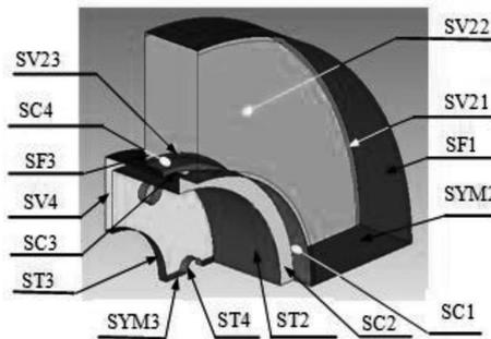
Fig. 6. Definition of surfaces of the full disc
