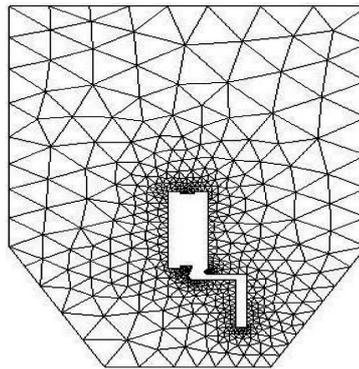
Fig. 8. Irregular mesh in the wall
