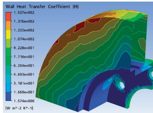
Fig. 10. Distribution of heat transfer coefficient on a full disc in the steady state case (FG 15)
