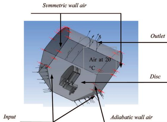
Fig. 9. Brake disc CFD model
