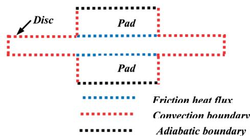
Fig. 18. Thermal boundary conditions applied on disc brake
