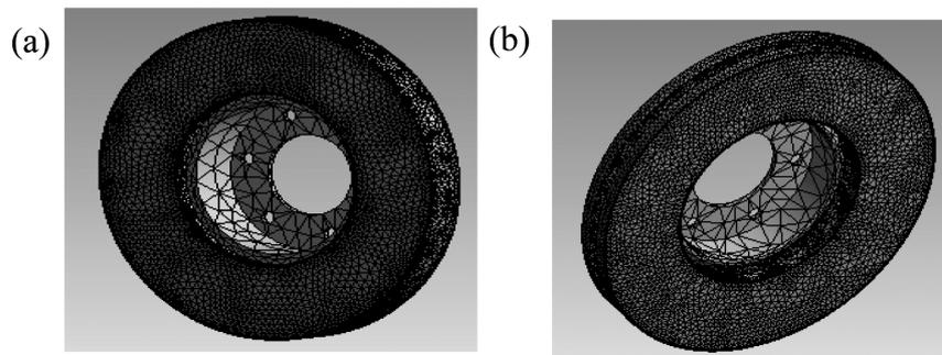
Fig. 16. Meshing of the disc (a) full disc (172103 nodes -114421 elements) (b) ventilated disc (154679 nodes- 94117 elements)
