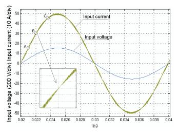
Fig. 4. Waveforms of mains voltage and mains current at the load of 7.8 kW
