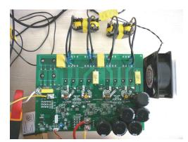
Fig. 10. Power circuit of the four-phase IPFC
