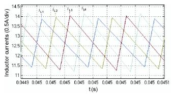
Fig. 7. Partial waveforms of four-phase inductor currents
