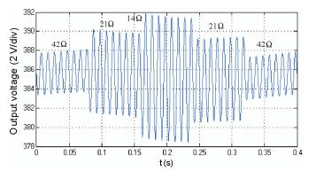
Fig. 9. Waveform of DC output voltage at different loads
