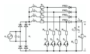
Fig. 1. Power circuit of the typical four-phase IPFC
