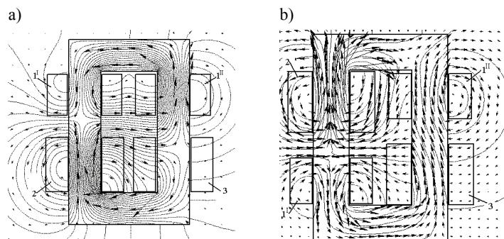
Fig. 6. The leakage fluxes of the transformers 1-2
