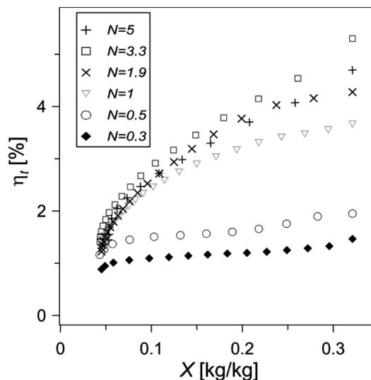
Fig. 4. Exergetic efficiency for different values of inlet air velocity
