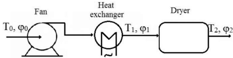
Fig. 1. Scheme of drying node
