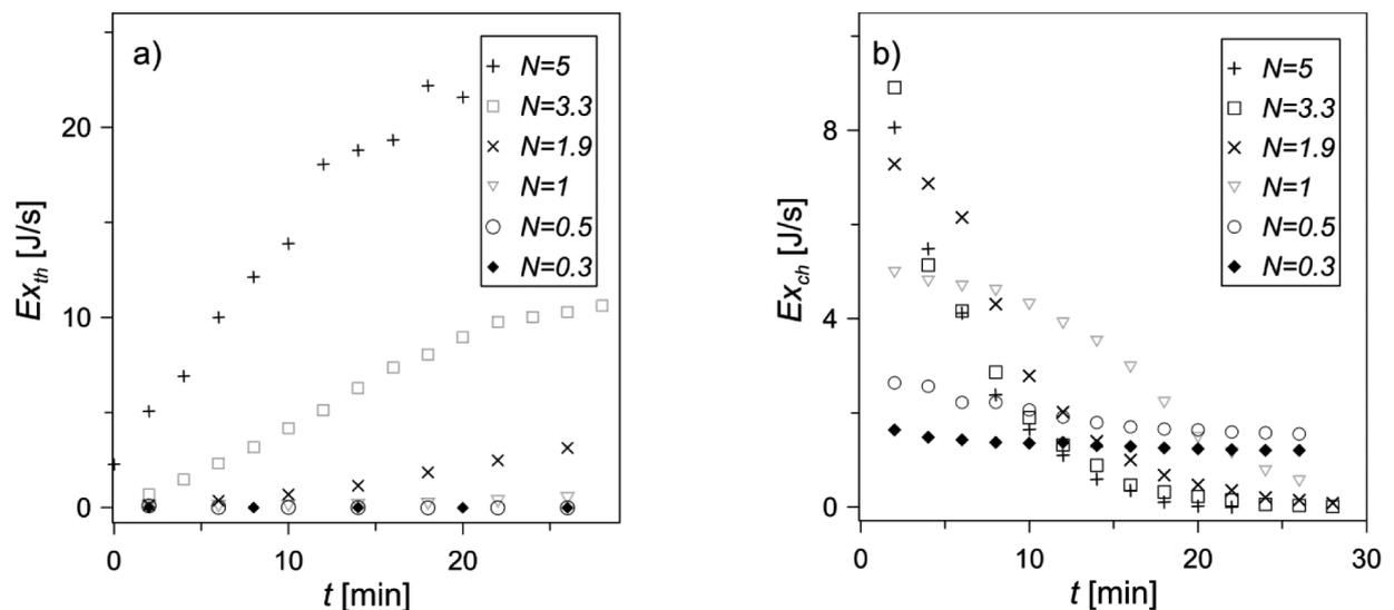
Fig. 9. Stream of: a) thermal exergy, b) chemical exergy of exhaust air versus time
