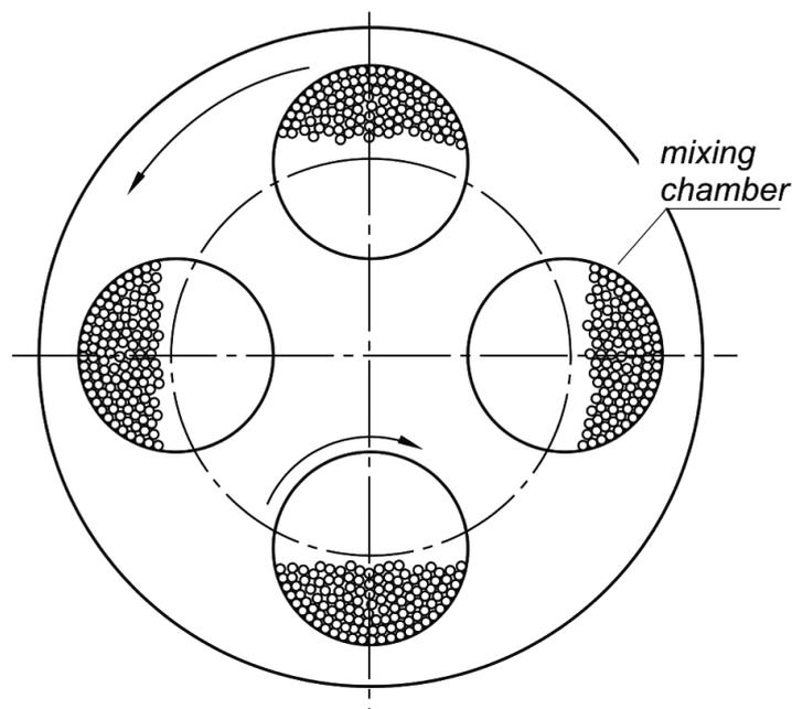
Fig. 2. Schematic representation of planetary ball mill
