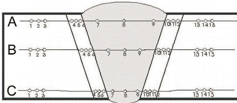
Fig. 6. Arrangement of hardness measurement points in welded joint
