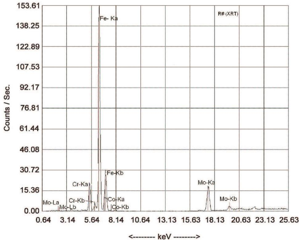
Fig. 10. X-ray radiation spectrum of PB2 weld
