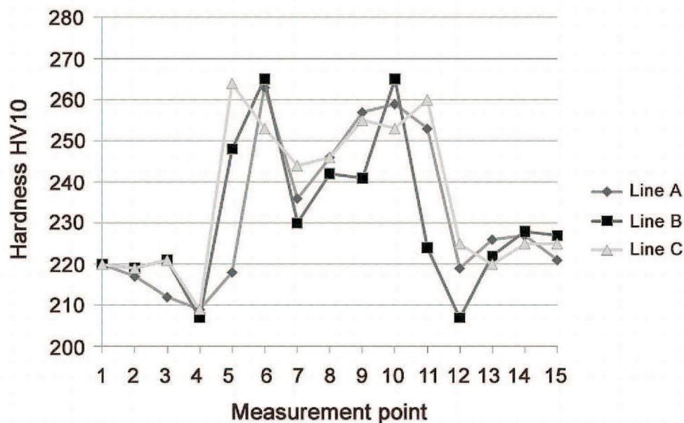
Fig. 7. Distribution of hardness in cross-section of welded joint of pipes ( $\phi$  219.1×31 mm) made of PB2 steel
