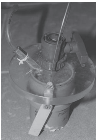
Figure 1. Apparatus for testing hydraulic conductivity with a sample of hardening slurry as tests are performed
