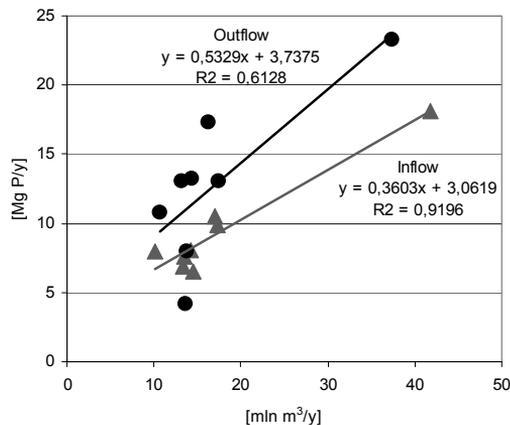
Fig. 4. Correlation between the amount of entering and leaving water and phosphorous load in the Plawniowice reservoir in the period 2004–2011
