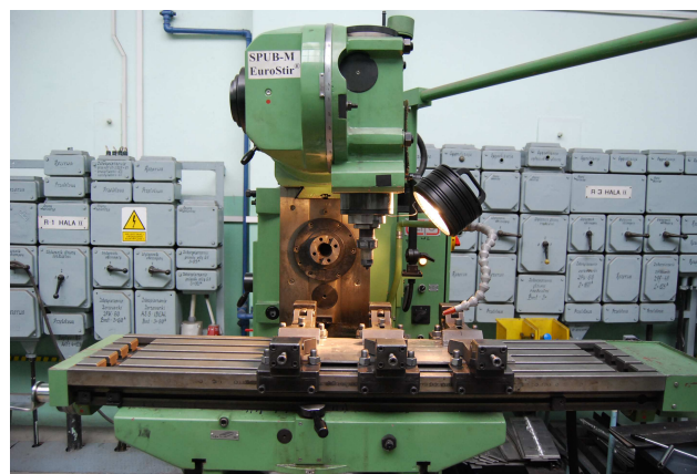
Fig. 1. General description of FSW method: a) the principle of FSW welding, b) welding station built in Instytut Spawalnictwa in Gliwice
