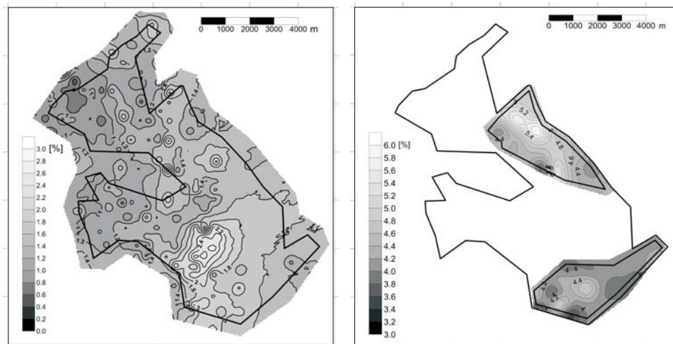
Fig. 4. The models of sulfur content distribution S_r^d in the lignite of seam II (left) and lignite seam IV (right) within the limits of the proposed operation
