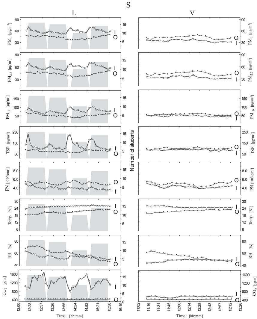
Fig. 2. Indoor (I) and outdoor (O) particle mass (PM) and particle number (PN) concentration, air temperature (Temp), relative humidity (RH) and CO<sub>2</sub> concentration time series in the occupied (L) and unoccupied (V) classroom C1(1) during one school day in the summer season (S) measurements
