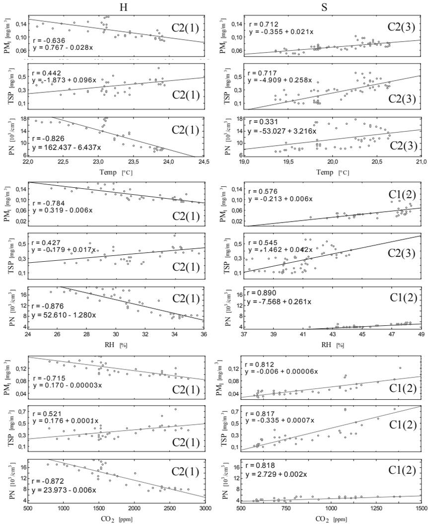
Fig. 3. The relation between the particle mass (PM1 and TSP), particle number (PN) concentrations and indoor air temperature (Temp), relative humidity (RH) and CO2 concentration in the occupied classrooms in the heating (H) and summer (S) seasons
