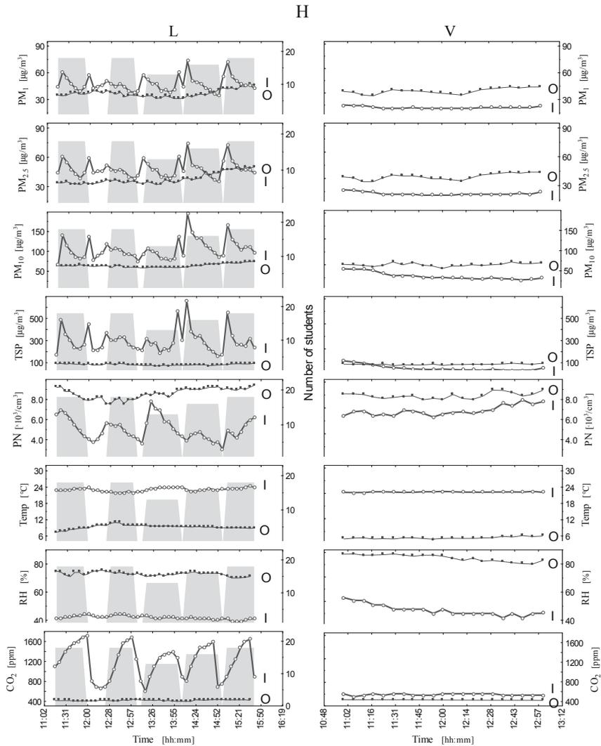
Fig. 1. Indoor (I) and outdoor (O) particle mass (PM) and particle number (PN) concentration, air temperature (Temp), relative humidity (RH) and  $\text{CO}_2$  concentration time series in the occupied (L) and unoccupied (V) classroom C1(1) during one school day in the heating (H) season measurements
