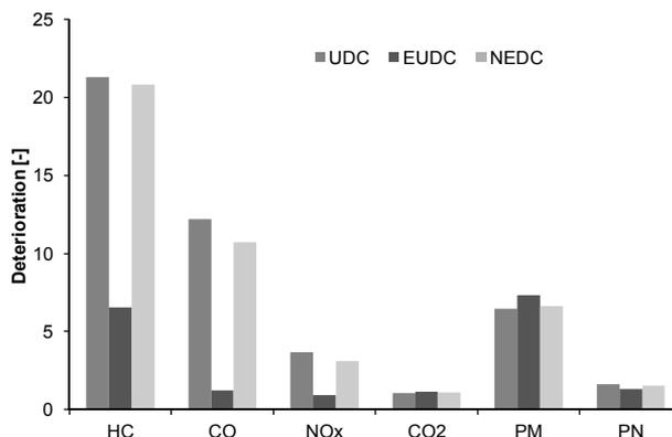
Fig. 7. Deterioration factors for a DISI vehicle tested over the NEDC at 24°C and at -7°C
