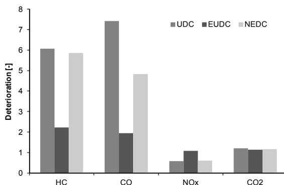
Fig. 6. Deterioration factors for a MPI vehicle tested over the NEDC at 24°C and at -7°C
