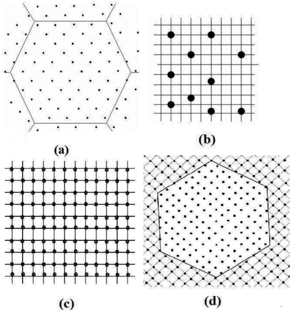
Fig. 1. Correlation of boundary-particles in a) random approach for coarse grained materials, b) non-random approach for nano-crystalline materials, c) stagnant of non-random approach predicted by Hillert [28] and d) abnormal growth in a nano-grained matrix
