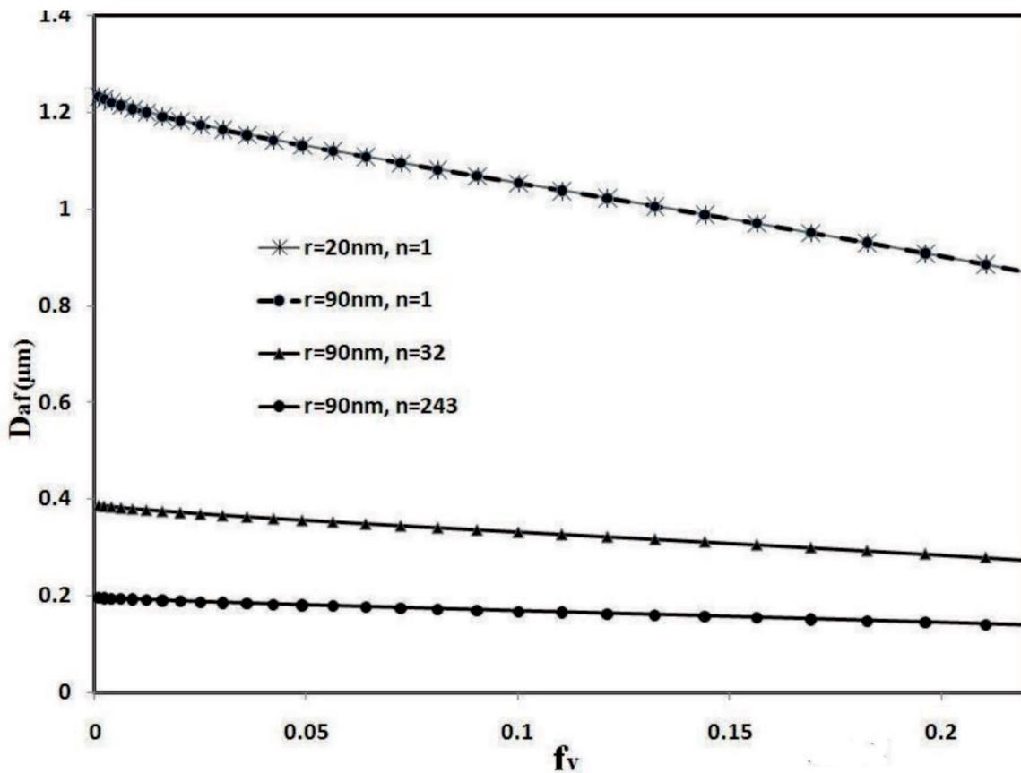
Fig. 3. Effect of volume fraction of nano-particles on the final size of abnormally growing grains
