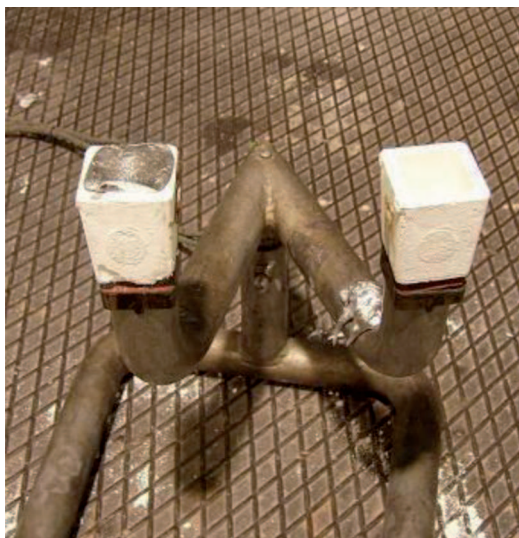
Fig. 2. Plaster cups mounted on the data acquisition device, the aluminium alloy has already been cast into the cup on the left
