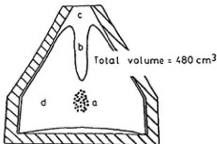
Fig. 6. a) microporosity, b) pipe volume, c) slumping and contraction volume, d) actual casting volume
