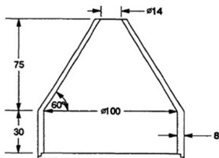
Fig. 7. Dimensions of tatur test (mm)
