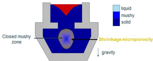
Fig. 5. Schematic illustration of a solidifying casted component with closed liquid pocket
