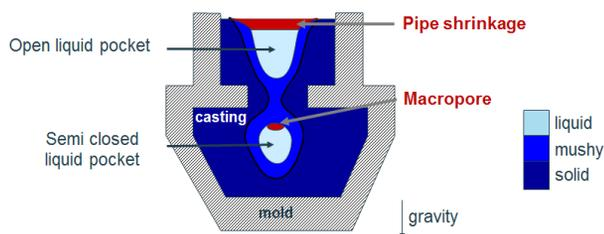
Fig. 4. Schematic illustration of a solidifying casted component
