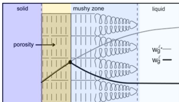
Fig. 2. Gas segregation in the liquid phase – gas solubility limit decreases with liquid pressure and temperature
