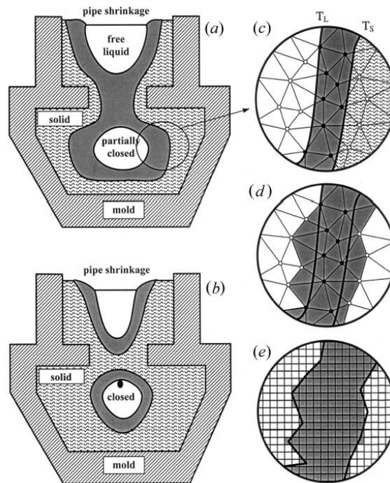
Fig. 3. (a) Schematic representation of pipe shrinkage at a top free surface and of a partially closed liquid pocket. (b) A macropore, which might start to form in a partially closed liquid region when this liquid region is closed. (c) A magnified view of the mushy zone shows that only a few FE nodes fall within its thickness (filled circles). (e) The FE elements are refined into small regular squares or cells (a), and those falling within mushy elements (gray elements in (d)) are activated.
