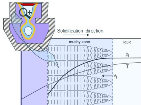
Fig. 1. Solidification shrinkage – liquid suction – liquid pressure drop in the permeable mushy zone
