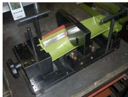
Fig. 1. Wax model of blade fixed in jig
