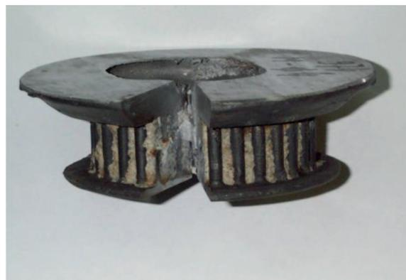
Fig. 2. The point of sample cutting from ingot top – filter poured with steel, for metallographic tests
