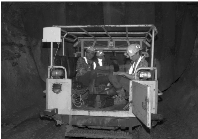
Fig. 6. Rx unit for WiMax 1,5GHz system mounted on car
