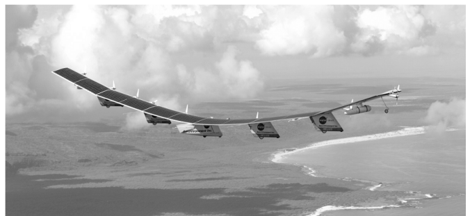
Fig. 4. Unmanned solar powered plane Helios [18].
