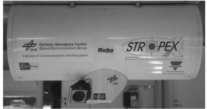
Fig. 8. Free-Space Experimental Laser Terminal (FELT) [3].
