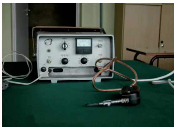
Fig. 2. Portable EIL-8A electro-spark deposition facility (TRIZ, Ukraine)
