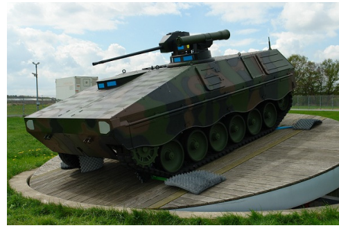
Fig. 4. Picture of the target: StanDCaM (Standard Decoy for Camouflage Materials), developed by WTD 52, Oberjettenberg, Germany. Surface material is metallized glass-fiber reinforced plastic.
